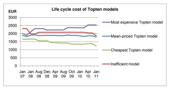
**Figure 6.** Life cycle cost of heat pump driers listed on <u>www.topten.ch</u> between 2007 - 2011 Assumptions: 1000 kg laundry dried per year, life span 15 years, electricity price 0.15 EUR/kWh<sup>7</sup>.
